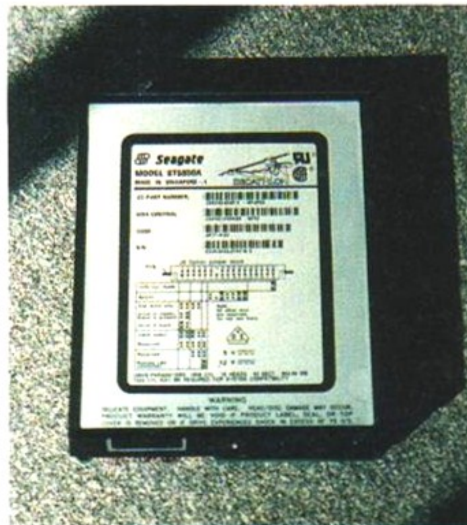
This Seagate hard drive has a table printed on it showing what the different jumper combinations do. It's a pity other drive manufacturers don't follow this example.
